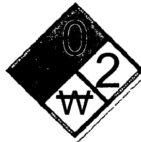
REQUIRED NFPA SIGNAGE
