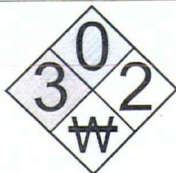
REQUIRED NFPA SIGNAGE
